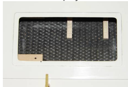
Glue with 5-min Epoxy
