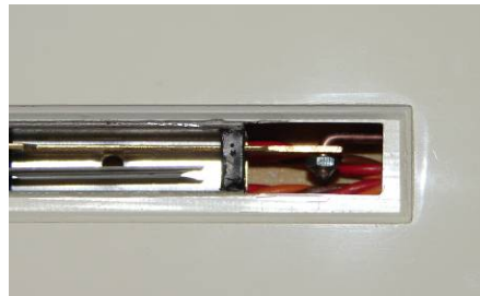
Fix the linkage with M2 nut and CA glue, strap up the hole with TESA® tape after completing
