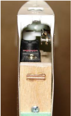
Screw the servo holder with two wood screws
