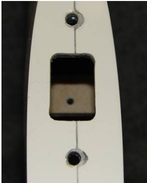
Glue the flanges for servo holder with 5-min Epoxy
