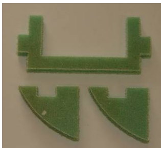
Holder for retract servo HS-75BB
