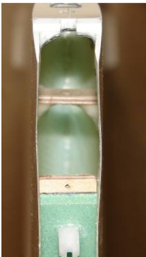
Glue the flanges for servo holder with 5-min Epoxy
